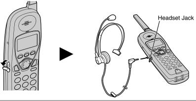
To switch to the speakerphone while using the headset:
