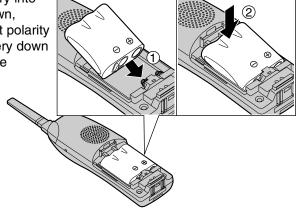
Glose the cover. Make sure you charge the new battery for about 15 hours in order to display the battery strength prompt correctly (p. 14).
