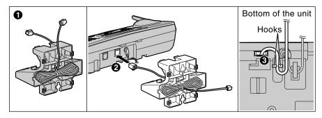
3 Insert (A) and (B) hooks on the wall mounting adaptor into the holes on the base unit.
